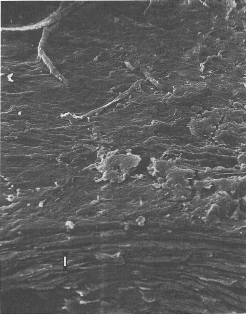
Figure 1. Scanning electron micrograph of cryofractured film containing 40% starch, 60% LDPE + EAA after 64 days of soil burial. Top of photo shows film surface; bottom shows film interior. Bar = 20 \mu\text{m} .
